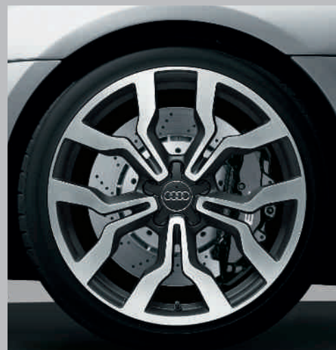
Forged aluminium wheels, 10-spoke Y design polished, two-tone, size 8.5 J x 19 at front, size 11 J x 19 at rear, with 235/35 R 19 tyres at front and 295/30 R 19 tyres at rear. (Standard for R8 5.2 FSI quattro)
