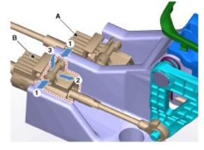
7. Remove the shift lever assembly (A) after removing the bolts.
