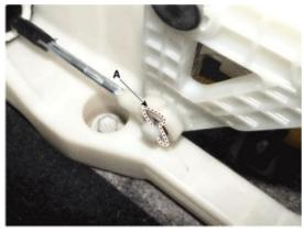
4. Remove the clip, in the shape of a "U"(B), from the cable end by spreading it towards both sides.
